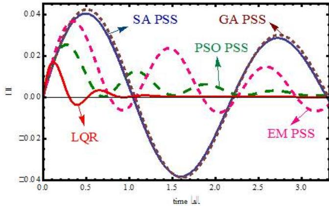
Figure 5: Single machine system response with different types of PSS for operating conditions "a"
