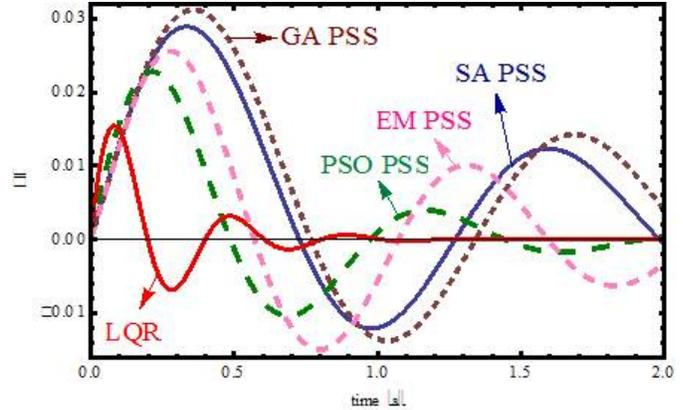
Figure 7: Single machine system response with different types of PSS for operating conditions "d"
