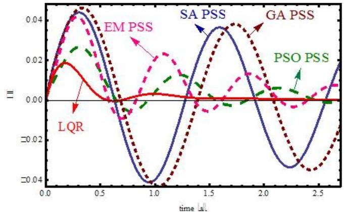
Figure 8: Single machine system response with different types of PSS for operating conditions "e"
