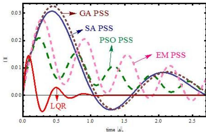
Figure 6: Single machine system response with different types of PSS for operating conditions "b"
