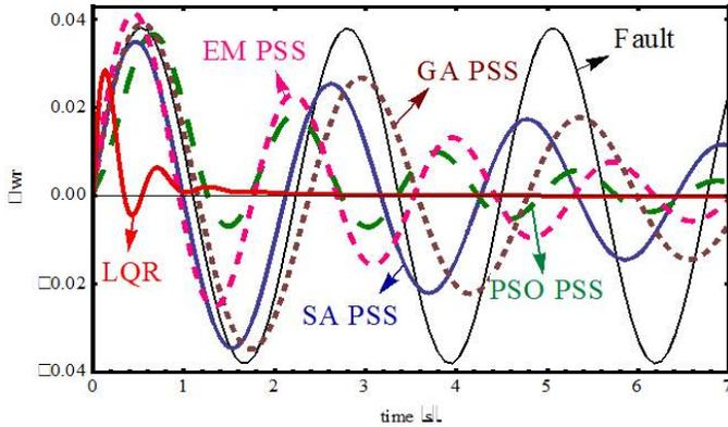
Figure 9: 10-machines system, G9 Response with different types of PSS
