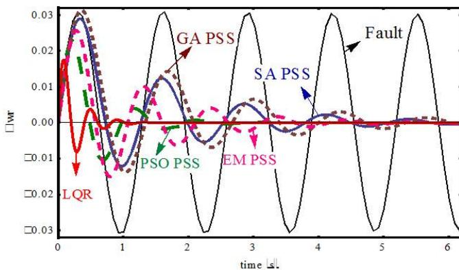
Figure 10: 10-machines system, G3 Response with different types of PSS
