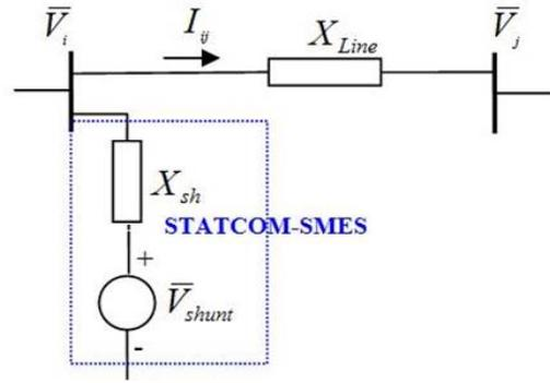
Figure 3: Equivalent circuit of STATCOM
