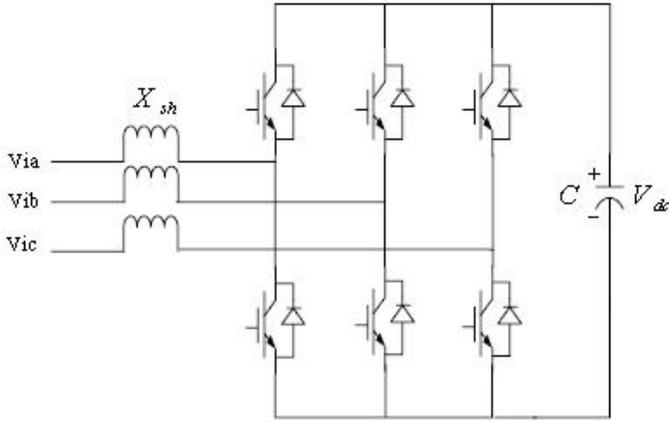
Figure 1: STATCOM schematic diagram
