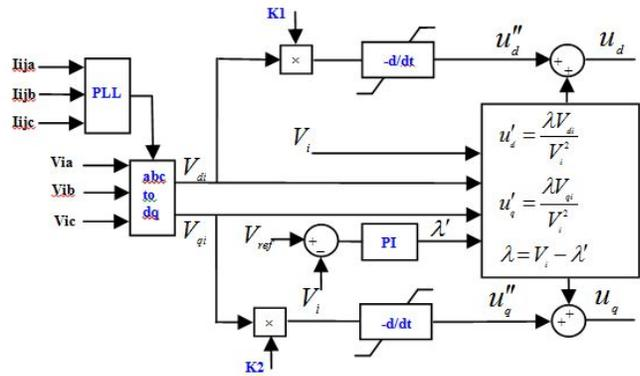
Figure 4: STATCOM control block diagram
